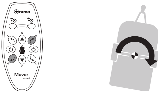
Fig. 28 ► After manoeuvring, apply the parking brake and/or secure the caravan with chocks to prevent it from rolling away first of all, then deactivate the manoeuvring system.
